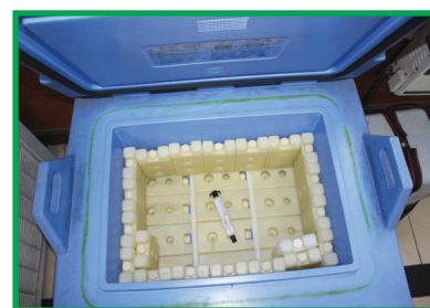
Cold box packed with icepacks and having a thermometer
